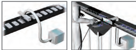
Removal of dust particles from mobile phone surface prior to painting with air blower & static elimination Collecting floating dust when air blowing adhered particles
