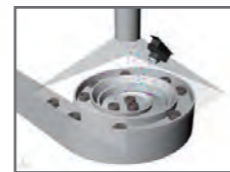
Collecting dust from parts feeder with static elimination
