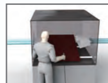
Removal of dust from car components with air blower
