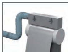
Removal of dust particles created by cutting lithium-ion battery electrodes
