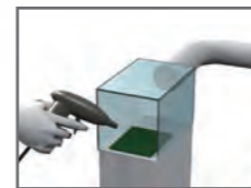
Removal of dust from circuit board with air blower
