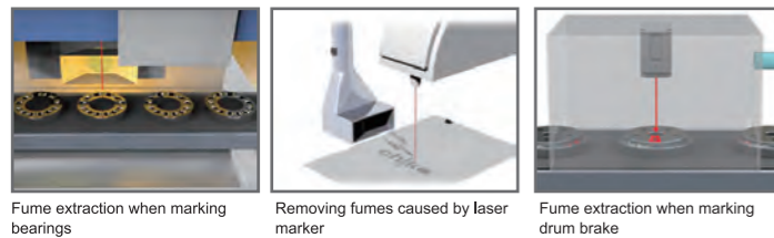
Fume extraction when marking metal workpiece
