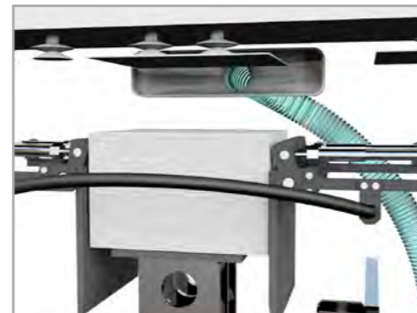
Removal of dust during the electrodes / separator conveying process
