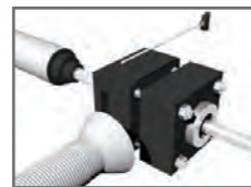
Removal of dust when molding with air blower
